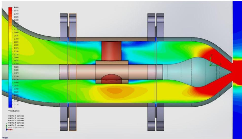
Fig. 8 – Velocity distributions (detail).
