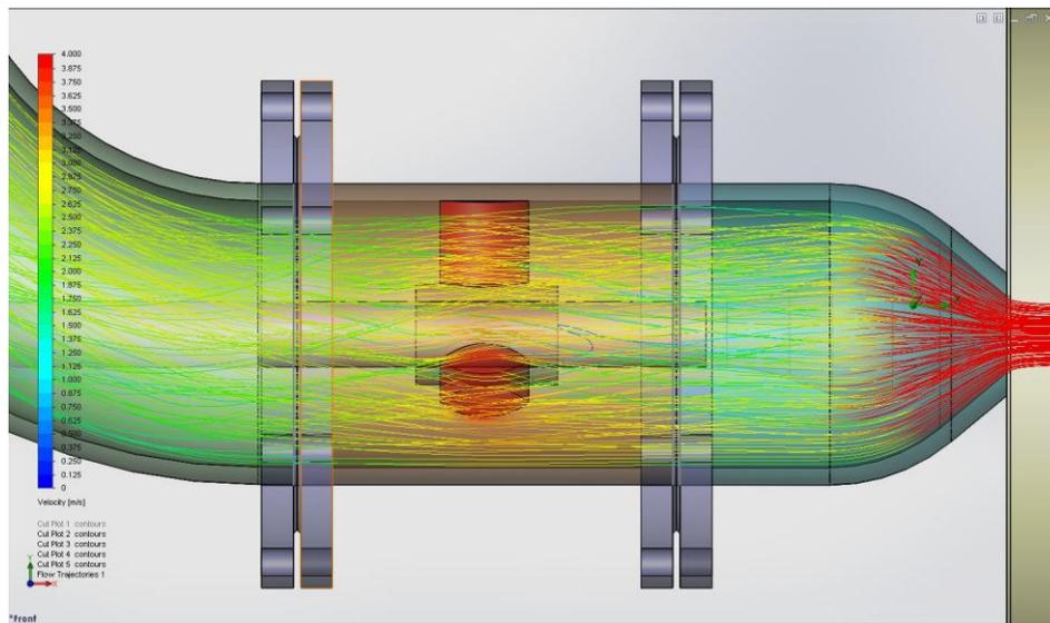
Fig. 10 – Streamlines (detail).
