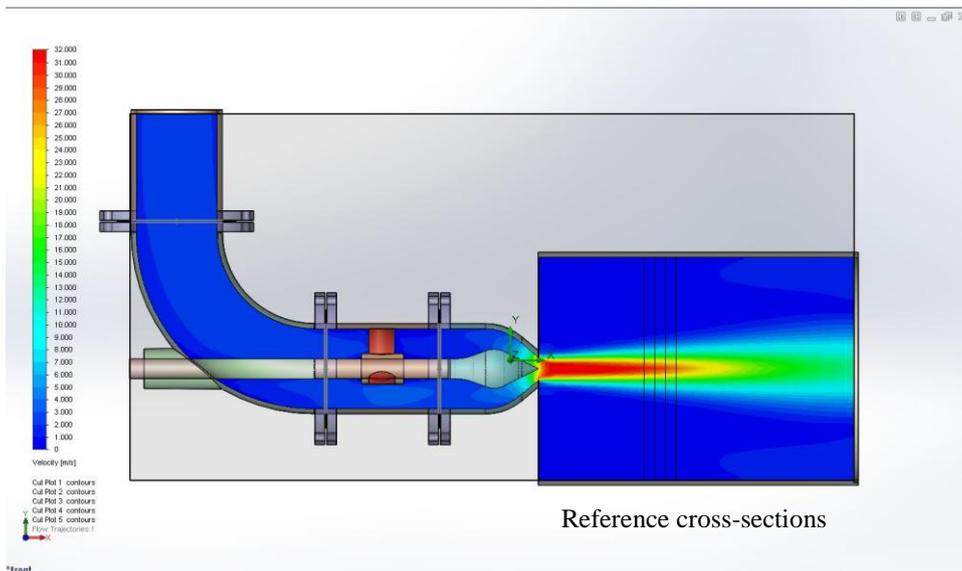
Fig. 11 – Position of reference cross-sections for velocity distributions at blade impact.
