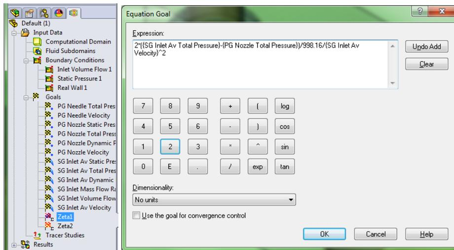
Fig. 6 – Pressure loss coefficient goal.
