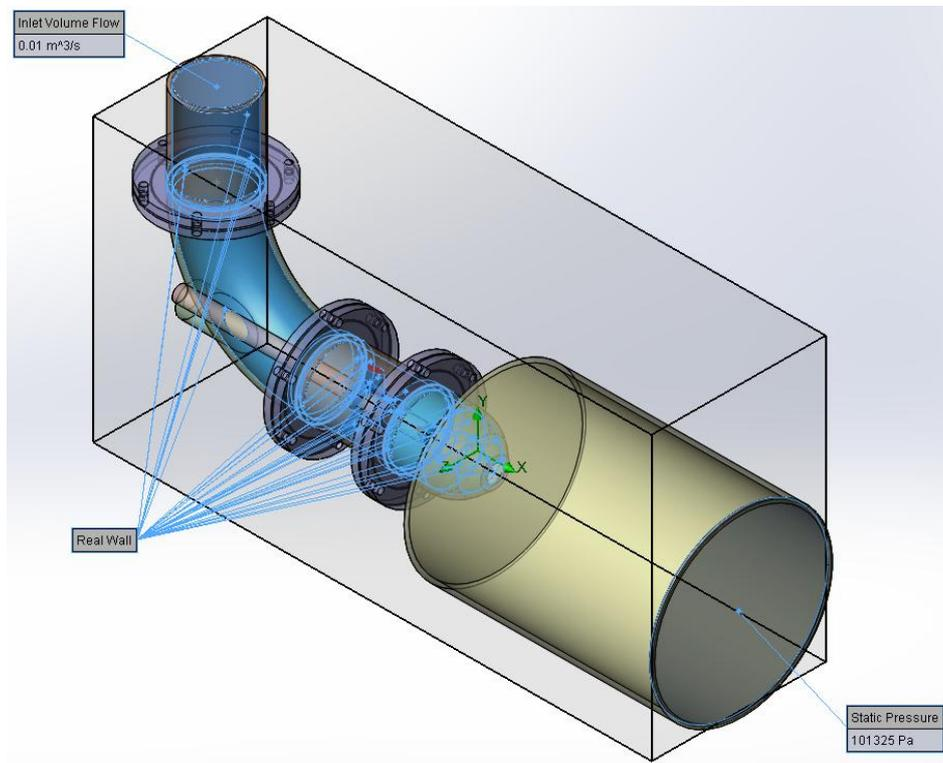
Fig. 5 – Inlet, outlet and wall conditions.
