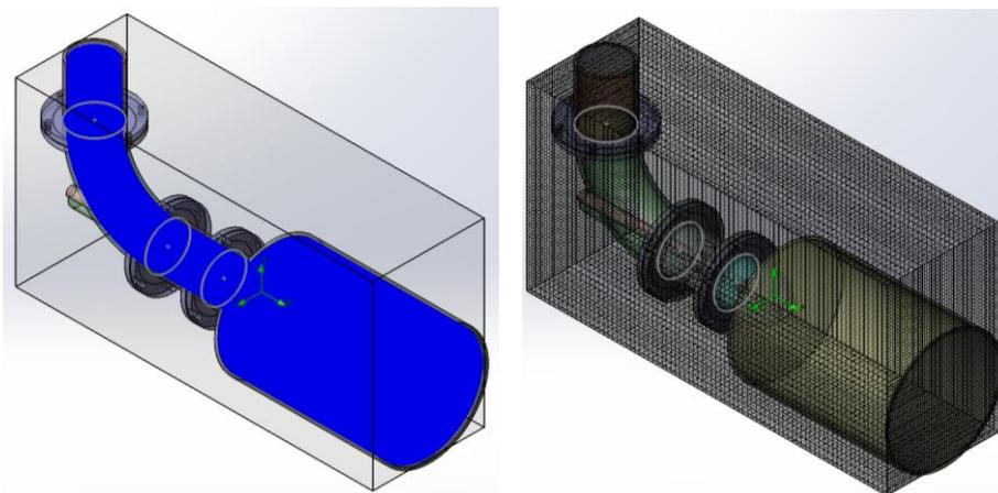
Fig. 3 – Flow domain and global mesh.
