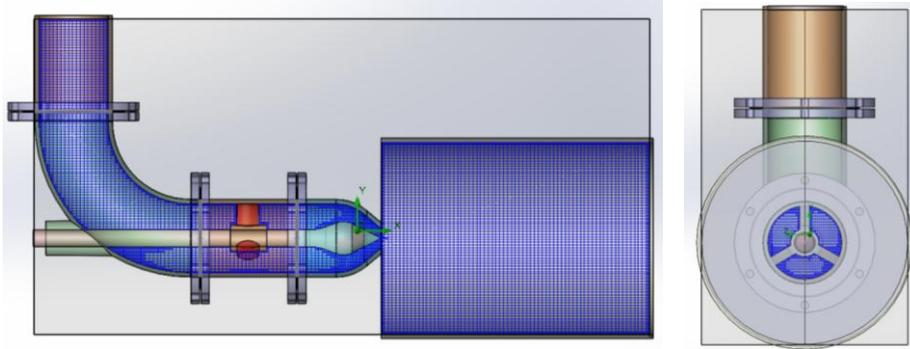
Fig. 4 – Fluid cells mesh in the main longitudinal and a cross-sections.
