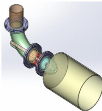
Fig. 1 – 3D-Model for the Pelton turbine nozzle and the hydraulic circuit.
